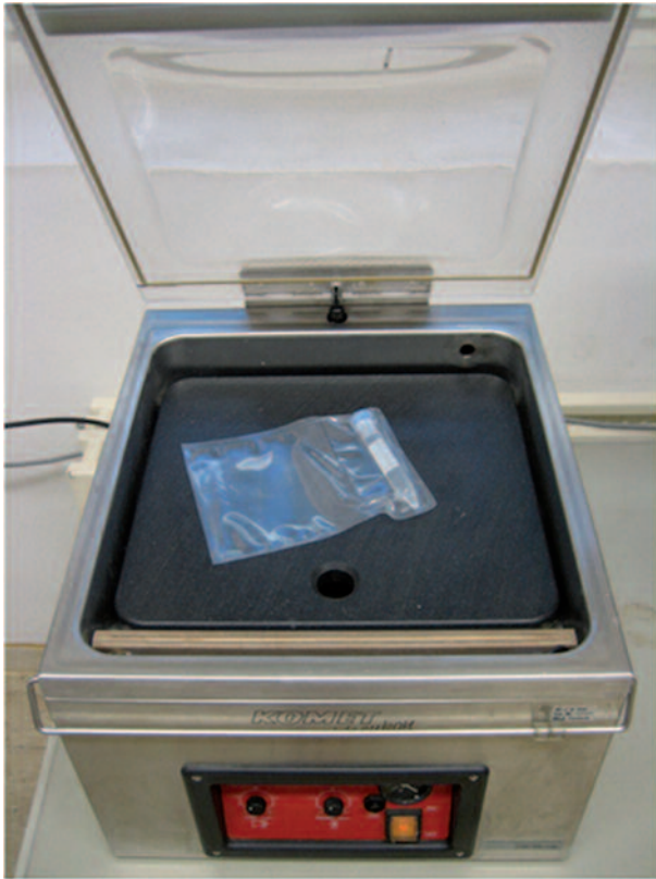
Figure 2. Vacuum sealing device (Komet, Plochingen, Germany). Specimens in polyethylene bags are placed into the vacuum chamber, positioning the open section onto the sealing bar. Once a vacuum is formed, a heated wire on the bar seals the plastic bag. On the control board, vacuum and sealing settings can be adjusted individually.
