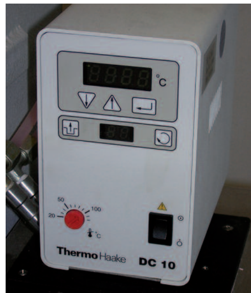
Figure 4. Temperature control unit (Thermo Fisher Scientific, Karlsruhe, Germany). Open-bath circulator with digital settings, bath vessel and bath bridge made of stainless steel and temperature resistant polymer; electronic control using a digital sensor for predetermined reference value, max. temperature 100°C.
